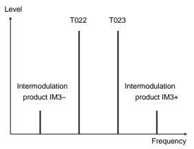
Figure 4: The 3<sup>rd</sup> order intermodulation products occur principally at the frequencies
