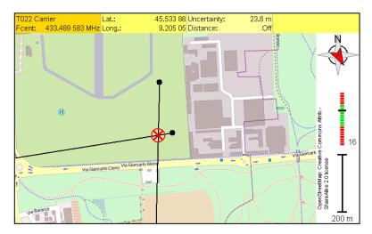
The cause of the problem is thus identified, so corrective measures can be taken. In this particular situation, only a reduction in the transmitted power will help. Technically, of course, steeper channel cutoff filters would be advantageous. Still, this technical effort can be spared by appropriately instructing personnel and by placing the transmitters further apart to avoid similar interference occurring at future events.
