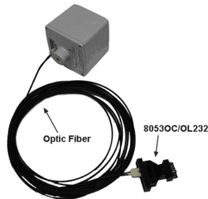
Fig. 4-3 EHP-200/A link with 8053-OC
