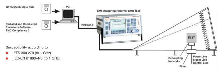
Fig. 12: Typical Test Set-up for Automotive Immunity Testing
