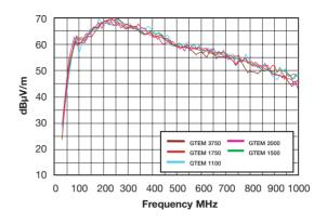
Fig. 9: Comparison of different OATS to different GTEMs (Source VSQ 1000, comparison of the emission measurement results of different open area test sites and different GTEMs)
