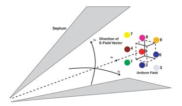
Fig. 5: Uniform field in GTEM 1500 (for E = 10V/m OdB = 35dBm (approx. 3 Watts CW)
