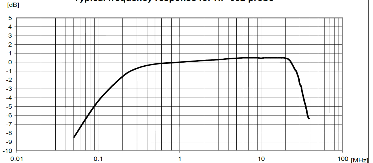
Typical frequency response for HP-032 probe
