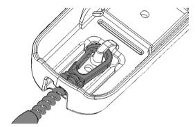
**NOTE:** By releasing the carabiner, the monitor can easily be removed from the mounting adapter. The monitor is then no longer protected against falling down, however!
