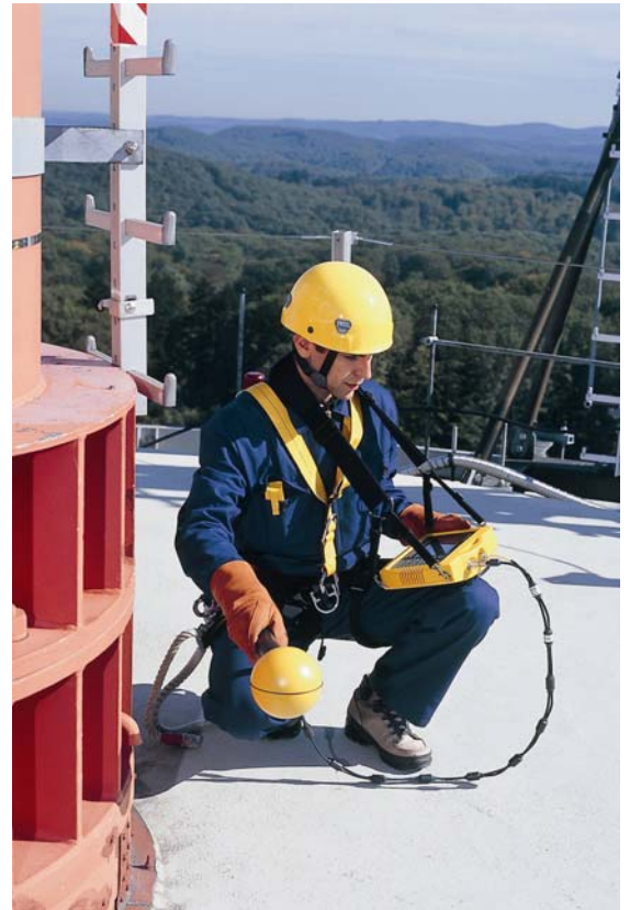
Spatial Averaging with the SRM-3000 and an isotropic E-field antenna.
