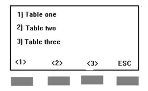
The above display examples shows the case where three different tables have been loaded. The name of the tables 1), 2) or 3) have been transferred from our software automatically. You can not change them from PMM3000 keyboard.
