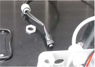
Connect the provided power supply/battery charger.
