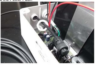
Plug the multipole battery charger connector to the Power pack
