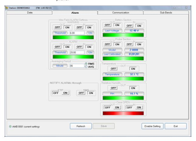
The same windows allows the user to set which average type should be performed on the acquired data, **AVG** or **RMS**, and the averaging period over which the average calculation is performed.
