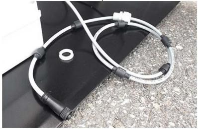
Install the power cable by mounting the chock in the hole of the receiver baseplate; plug the power supply connector to the receiver unit holding by the plastic part.
