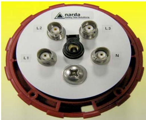
A-D-18 PMM L3-64 model adapter (64 A sockets)
