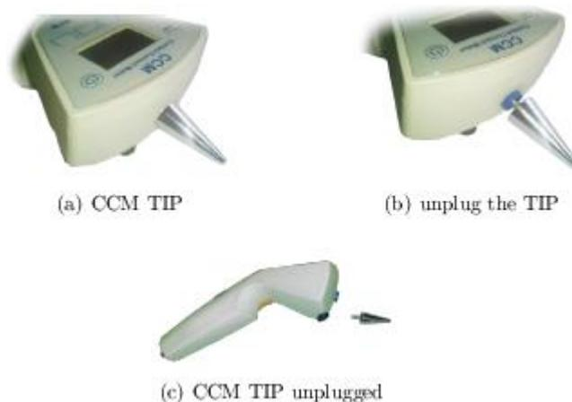
Figure 7-2. Remove the TIP
