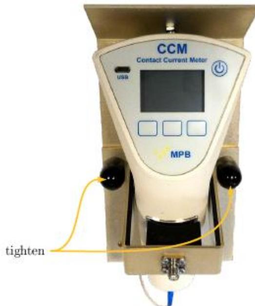
Figure 7-4. Set Up JIG
