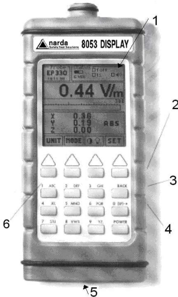
Fig. 10-4 Front panel
