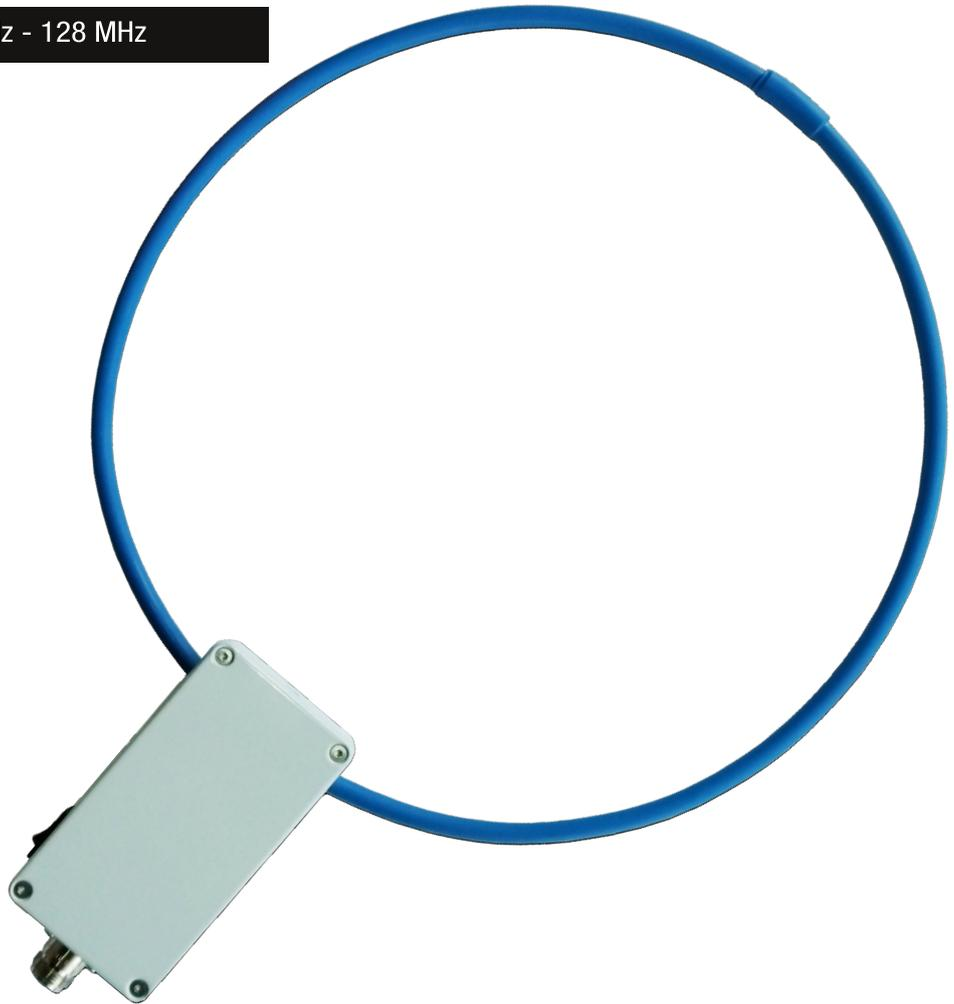
The L4-A is an active loop antenna for the magnetic component of the electromagnetic field for EMI or shielding effectiveness measures. It has a low noise preamplifier which increases overall measurement sensitivity. This antenna is powered by 4 AAA replaceable batteries (1.2 V or 1.5 V).
