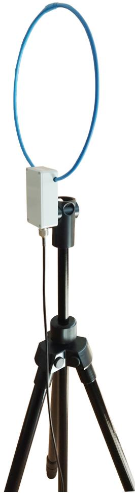
Through the 1/4" thread the L4-A active loop antenna can be easily plug on the NMR-01 amagnetic and non reflective tripod.
