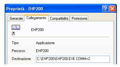
In some operating system the Destination field is enclosed in double quotation marks ("); in this case, the command COMM=N, preceded by a space must be outside as in the example below;
