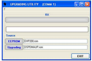
To start the process simply switch EHP-200/A on and wait (few minutes) until the automatic transfer is completed.
