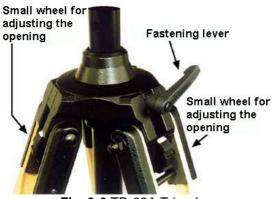
Fig. 9-6 TR-02A Tripod
