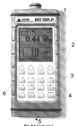
Fig. 9-4 Front panel
