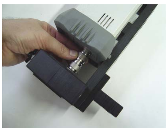
Fig. 11-14 Screwing the N-N Adapter for Antenna Matching
