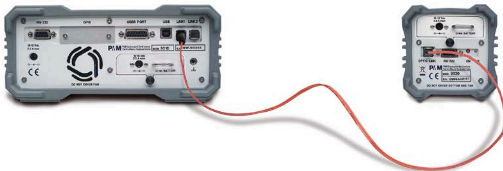
Fig. 11-5 PMM 9030/9060/9180 Fiber Optic Link to PMM 9010
