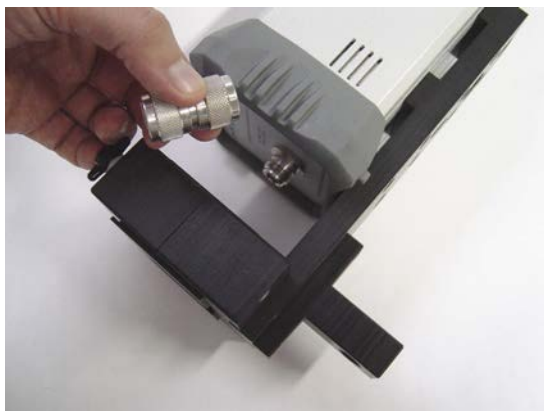
Fig. 11-14 Screwing the N-N Adapter for Antenna Matching
