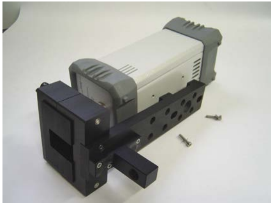
Fig. 11-13 Mounting the Antenna Holder on PMM 9030/9060/9180
