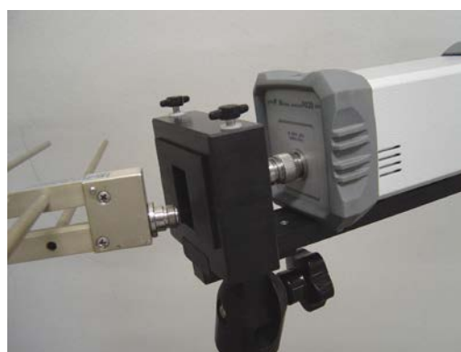
Fig. 11-16 Attaching PMM LogPeriodic
