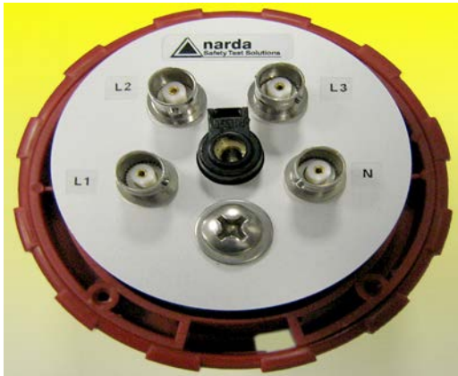
A-D-18 PMM L3-64 model adapter (64 A sockets)
