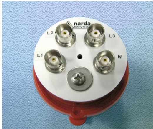
A-D-17 PMM L3-32 model adapter (32 A sockets)
