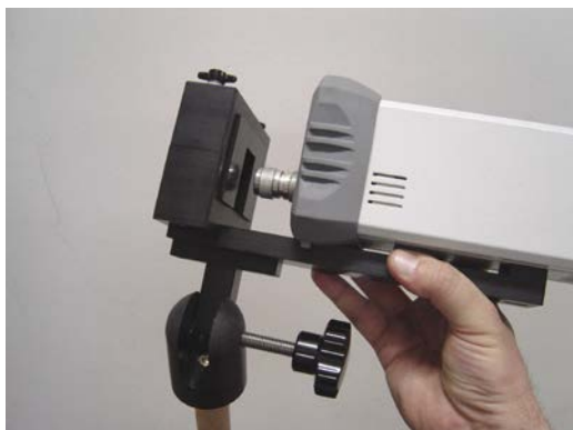
Fig. 11-15 Fixing onto the Tripod
