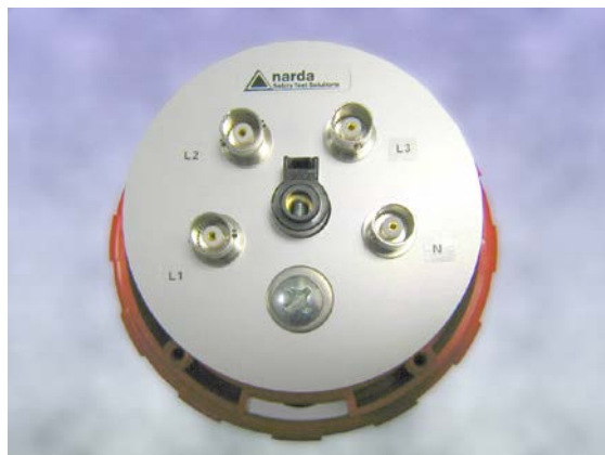
A-D-19 3-phase socket to BNC adapter. Model adequate to PMM L3-100 and higher (100 A sockets)
