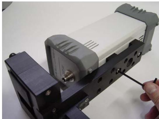
Fig. 11-13 Mounting the Antenna Holder on PMM 9030/9060/9180
